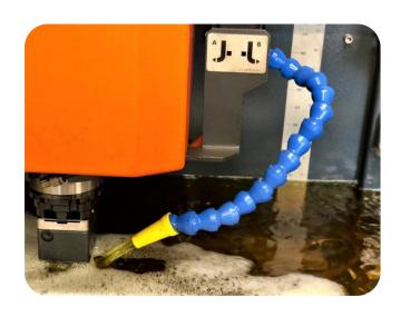
Whole system is manufactured form material POM which excels in hardness, dimensional stability, strength, wear resistance, low friction and low weight. System is are applicable in the temperature range from -40°C to 130°C. Compared to other plastic materials POM does not absorb humidity therefore parts are not breakable at low temperatures.
